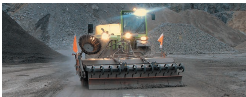
bema 75 Dual PowerMaster with scraper unit instead of collection container, rotary side brush, high pressure water unit and water tank in the rear (see page 58/59)
